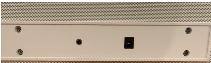
Figure 1 – Rear Panel Audio and Power Cable Connections
