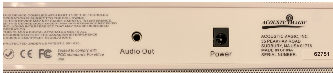
Figure 1 – Rear Panel Audio and Power Cable Connections
